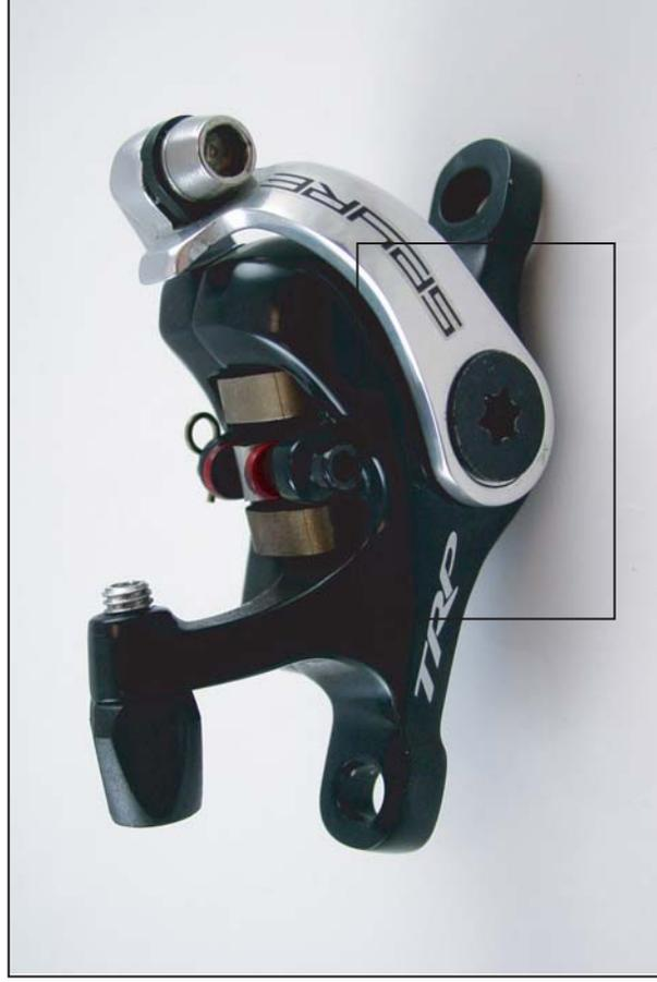
The old Spyre had a single pad adjust screw and did not have laser etch markings. The outside is marked with a Torx head.
