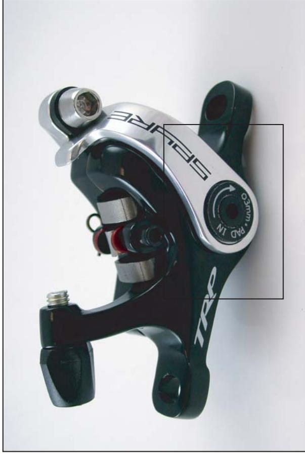
The new Spyre has a pad adjust on both sides of the brake. Using a 3mm hex wrench, the pad can be adjusted inward by turning clockwise.
