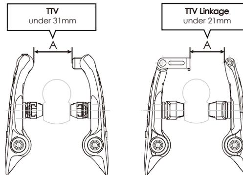
3.) Before finally tightening brake pads, make sure they are aligned correctly on the rim, and there is a gap of 1mm between the top of the rim and the top of the pad. Hold each pad against the rim (one at a time) & tighten mounting nut. **Final tightening torque: 6-8Nm.**
