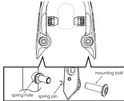
2.) With both pads pressed against the wheel rim, ensure that distance-A (in diagram) does not exceed 31mm or 21mm in linkage version. To increase distance-A, take off inner spacer on each brake pad.
