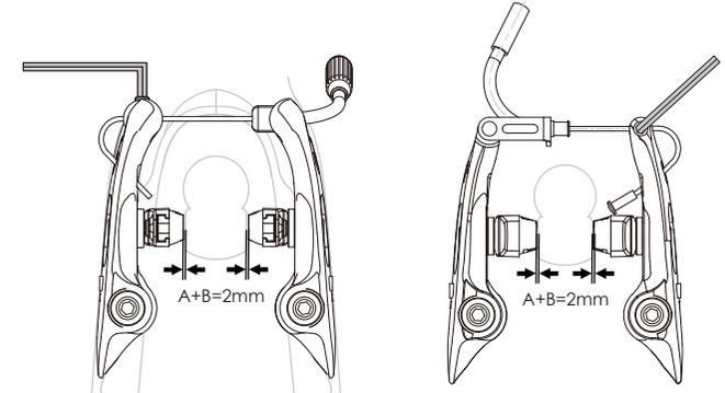
5.) Balance brake arms by turning spring-tension adjusters. Depress brake lever a few times while checking to see that tension is equal for both arms. Pad/rim contact should occur at the same time each side. Clearance should be 1mm each side. **Do not see tension too high.**
