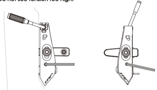
6.) Readjust pads so they are properly aligned (see Step3), as tension adjustment will probably have altered original pad alignment.
