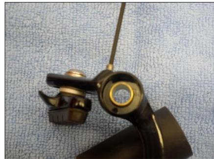
Tension Adjuster Plate – Blocking Adjuster Screw
