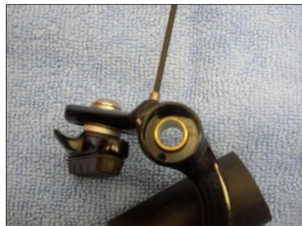
Tension Adjuster Plate – Blocking Adjuster Screw
