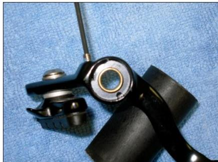
Tension Adjuster Plate – Correct Position
