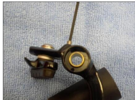
Tension Adjuster Plate – Blocking Adjuster Screw
