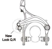
(2) Push the lock device and open the Q.R lever.
