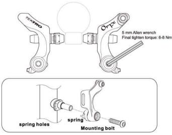
2.With both pads pressed against the wheel rim check that the inside edges of the brake arms are approximately parallel with the rim. Ensure that the brake arms are not diving into the rim. Before finally tightening the brake pads on the brake arm, make sure they are aligned correctly on the rim, and there is a 1mm gap between the top of the rim and the top of the pad. Hold each pad against the rim(one at a time) and tighten the mounting nut. Tighten to a final torque of 6-8 Nm.
