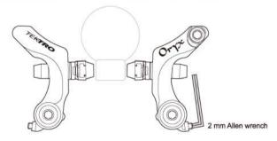
A note about brake pads, All Tektro pads have grooves running up and down on the pad/rim contact surface. Once these grooves have been worn down so they are no longer visible, the pads should be replaced. Continued use past the wear line could result in damage to your rim and inferior braking performance.
