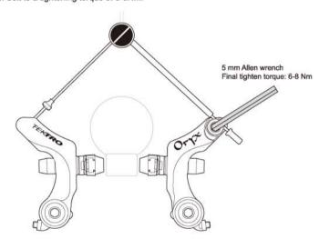
5.Balance the brake arm by turning the spring tension adjusters. Depress the brake lever a few times while checking to see that the tension is equal on both arms. Pad/rim contact should occur simultaneously on each side. Do not set the tension too high.
