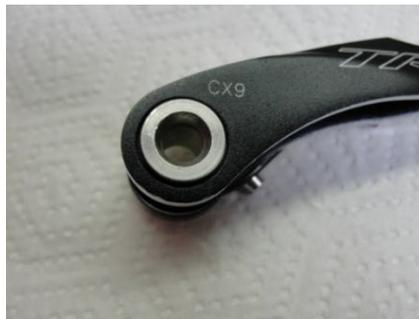
Apply an ample amount of grease to the bushing pivot barrel and reassemble the pivot bushing barrel and spring assembly.
