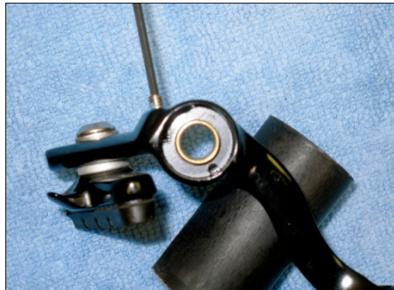
Tension Adjuster Plate – Correct Position
