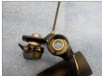
Tension Adjuster Plate – Blocking Adjuster Screw
